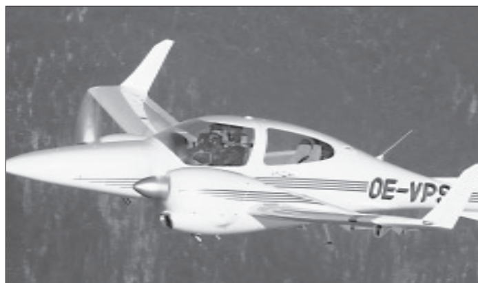
Diesel-powered twin-engine Diamond DA42, operated at maximum economy, a speed of 126.6 mph, gets what amounts to an astounding 42 mpg.
