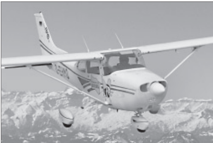
Cessna 172s are one of the aircraft to which the Centurion diesel has been retrofitted. One of the test aircraft registered fuel economy of 27.4 mpg at 126.6 mph.
