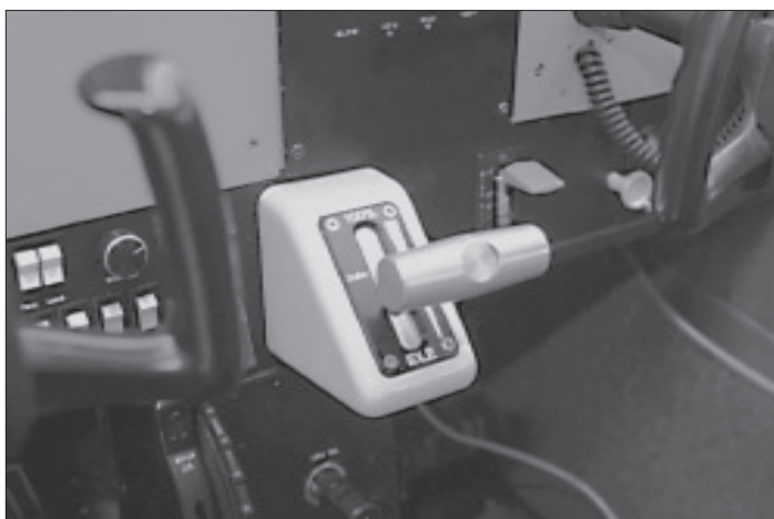
One knob does it all in aircraft powered by the diesel Centurion. There is no fiddling with mixture control or carburetor heat.
