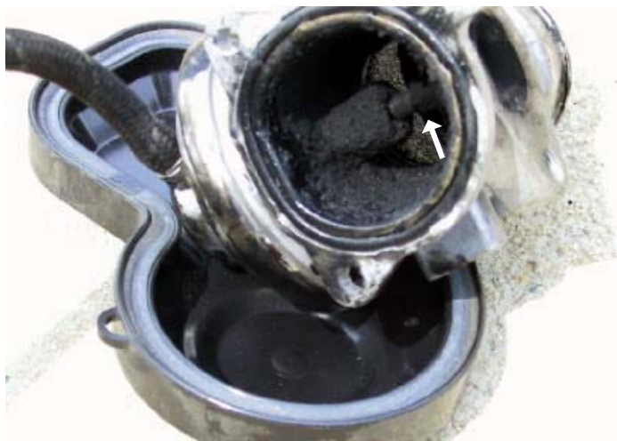
Crankcase vented oil mixes with EGR. The arrow points to the EGR valve. Your 2004 Cummins engine will have EGR but will not have the vent oil introduced into the clean intake air.
