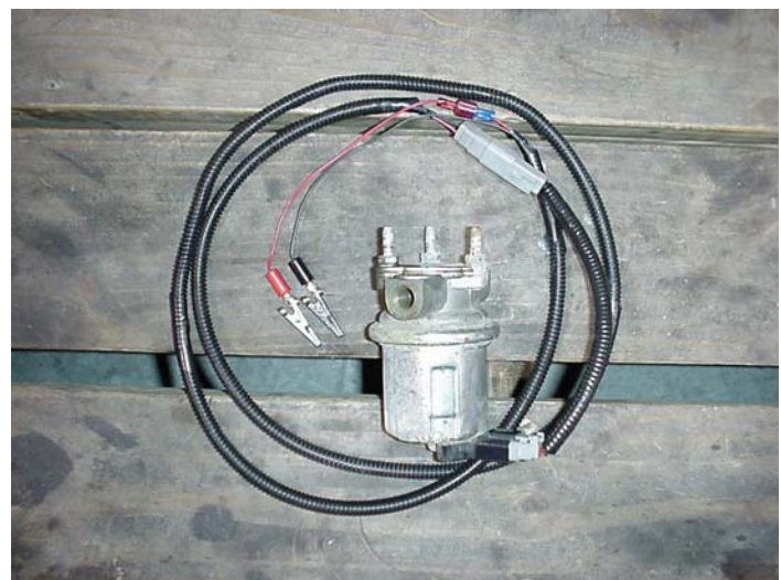
Another shop trick: testing a 24-valve fuel delivery pump is easy with the correct wiring harness and jumper leads that go directly to a 12-volt battery.
