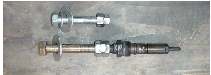
This is an innovative shop tool developed by TST to remove 12-valve injectors.
